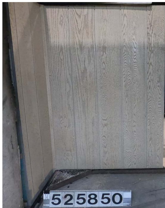
Figure 7: Total view of the exposed surface of the long wing prior to testing
